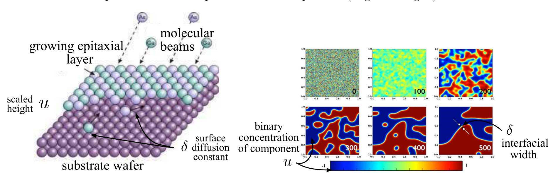
Figure 1: MBE (left): thin film epitaxy; CH equation (right): phase separation
